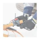
1. Turn the locking knob to loosen the control block clamp from the PORT-A-TROWEL handle connection adaptor, slide the control block upwards and remove from the handle.
