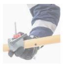
2. With the control block removed from the PORT-A-TROWEL slide the orange painted end of the clip together handle through the control block. Slide the control block so that is sitting approx.. half way along the handle (900mm from either end) – Tighten the control block into this position with the locking knob.
