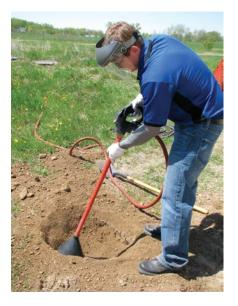
The Soil Pick requires no periodic maintenance. A pressure gauge on the handle assembly advises the operator if the tool is working at acceptable pressure. The Soil Pick weighs 6.2 lbs., has zero hand/arm vibration and can be used for extended periods without fatigue.
