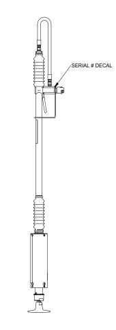
The unit's serial number can be found on the decal located on the Handle Assembly.
