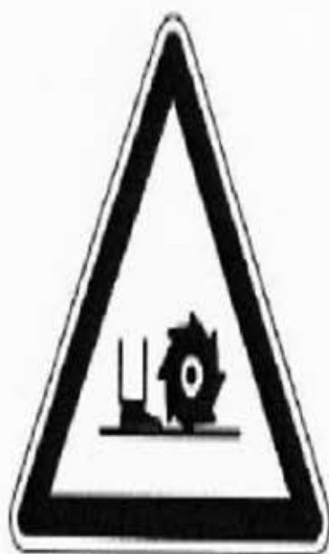
Danger: risk of cut
